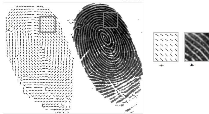
Figure 4: Orientation fields of a fingerprint image (109-5 DB1 FVC2004) after histogram equalization with W=10 . -a- orientations in an homogeneous block -b- original image in the block
