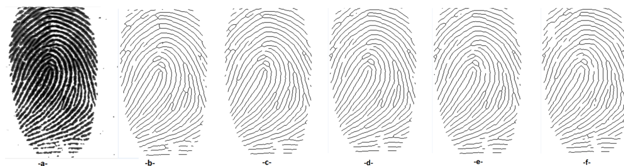
Figure 3: a-Original fingerprint image 103_1 of DB1 FVC2004,after histogram equalization, -b- Thinned fingerprint output after processing FFT \times |FFT|^k with k=0.30 , -c- with k=0.45 , -d- with k=0.55 , -e- with k=0.85 , -f- with k=1 .
